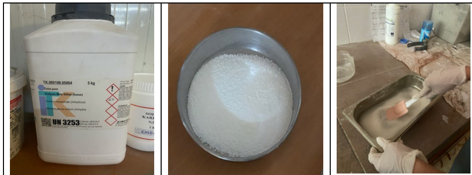
Figure 3: Solid activator and dissolution of the solid activator in water
