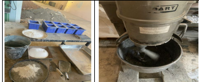
Figure 2: Cube specimens and materials in Hobart mixer
