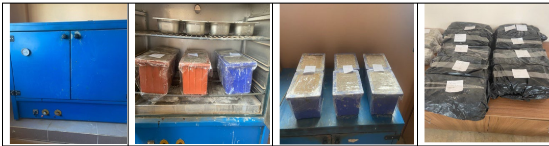
Figure 5: Experiment furnace, placing concrete samples to furnace, samples after furnace and samples waiting for test day
