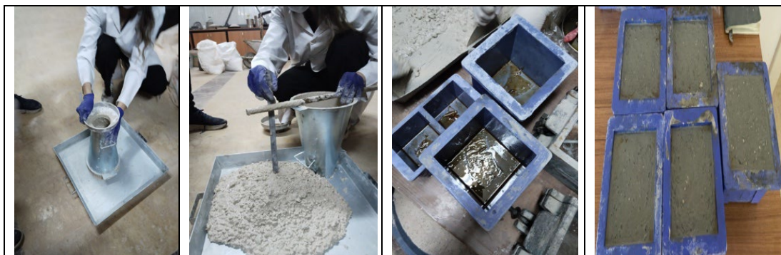
Figure 4: Slump test and placing concrete to molds
