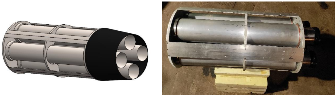
Figure 3: Four RM-12K motors arranged in a parallel configuration propulsion unit.
