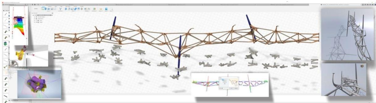
*Figure 6. Autodesk InventorPro/Fusion360 Topological Optimizations (TO) of the nodes and entire geometry, with RFEM tests in Dlubal and Dynamo-Grasshopper. Renderings in Autodesk-Maya-Alias. Source:© Thomas Spiegelhalter. .*
