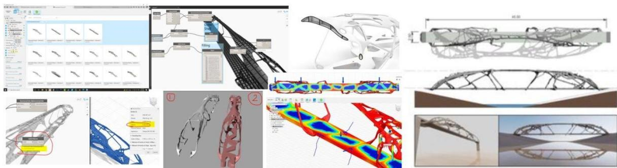
Figure 3: Autodesk InventorPro/Fusion360 Generative Design with organic experimental GA/EA workflows and Dynamo Scripting to topologically optimize the weight and material choices for fabrication. Source:© Thomas Spiegelhalter.
