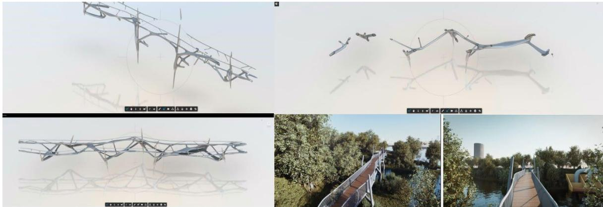
Figure 5. Autodesk InventorPro/Fusion360 Generative Design and Topological Optimizations (TO) with genetic and evolutionary Algorithms (GA/EA), SIEMENS NX, Dynamo Studio. Renderings in Revit. Source: © Thomas Spiegelhalter.
