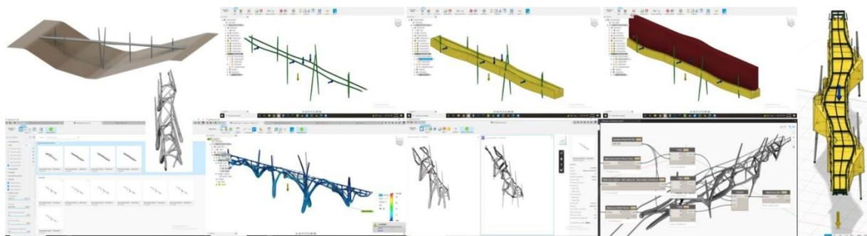
Figure 4: Autodesk InventorPro/Fusion360 Generative Design space, constraints, obstacles, offsets, with genetic and evolutionary Algorithms (GA/EA) and Dynamo Scripting. Source:Source:© Thomas Spiegelhalter.
